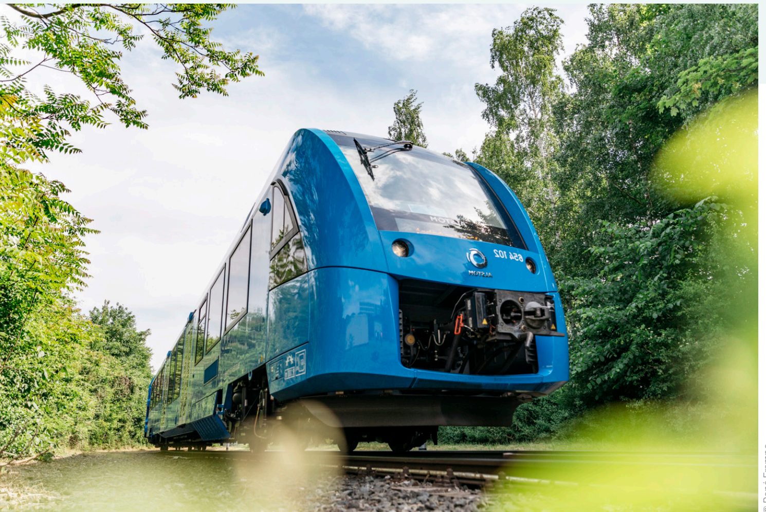
Coradia iLint, first hydrogen fuel cell powered train developed by Alstom for Germany
